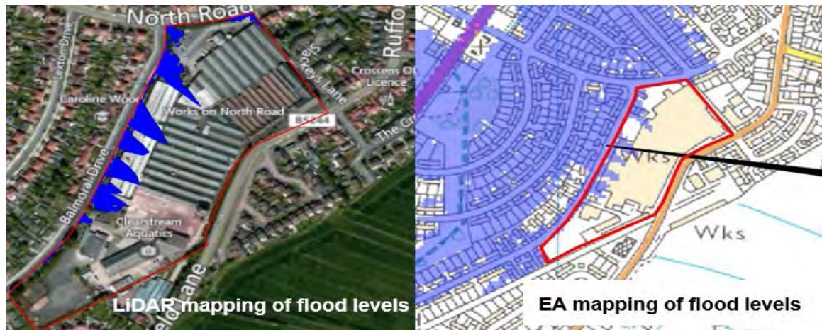
Figure 3: Comparison of Flood Extent between Contoured LiDAR data and EA Breach Mapping
